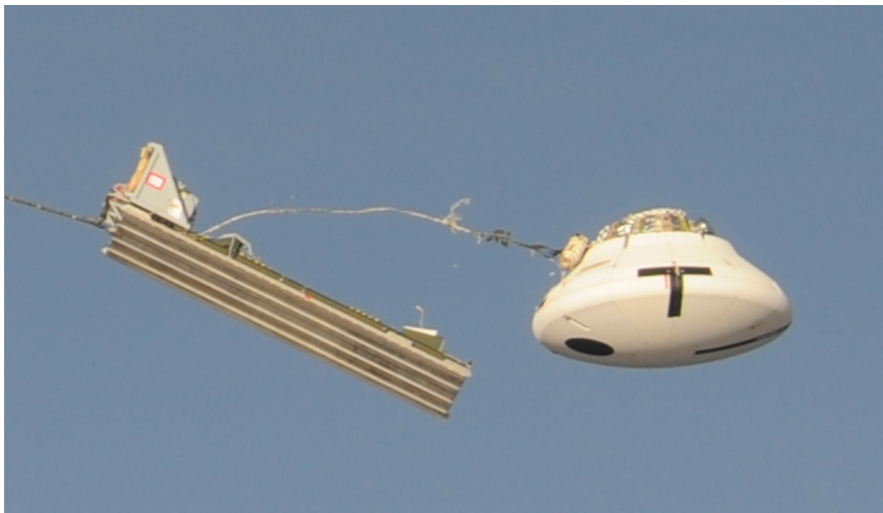
Figure 2. Photograph of the PTV separating from the CPSS and Programmer parachute deployment.
